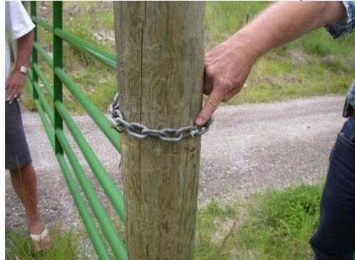
To release/open gate simple give a good push by hand to the gate thus breaking the wire tie
